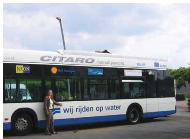
Fig. 2 Wij rijden op water (we ride on water) is the motto on this fuel-cell hydrogen bus used for public transport in Amsterdam. Actually, the bus is fuelled by hydrogen generated from electrolysis of water.
